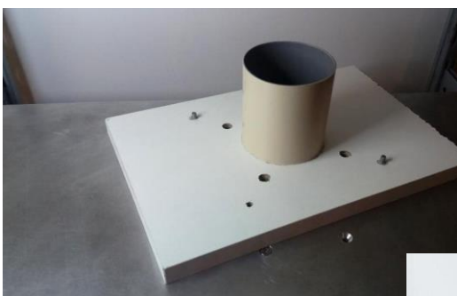
Figure 6 Bottom with locating dowels
