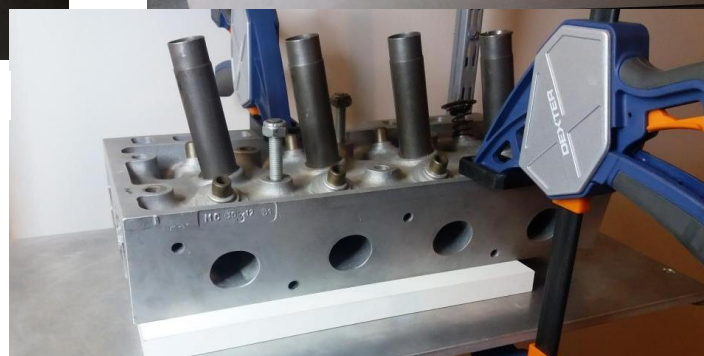
Figure 7 Assembly of the cylinder head with centering bolts
